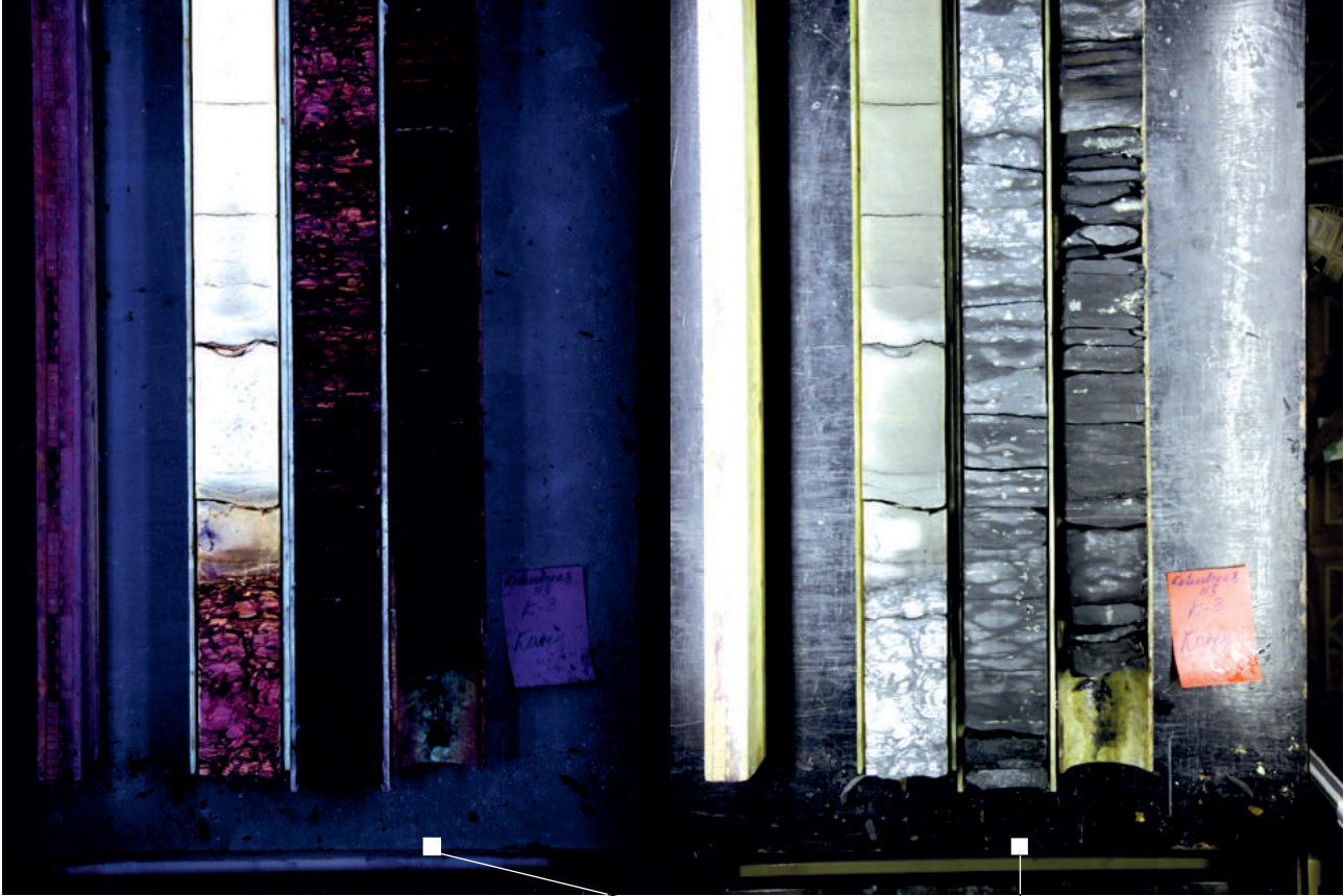
▲ Core luminescence. Oil-saturated sandstone interval. Well No. 9. Blue core luminescence is typical for marine sedimentation sandstone (which indicates that there are no significant hydrocarbon clusters), blue-yellowish luminescence is typical for lagoonal sandstones (which indicates their productivity).
