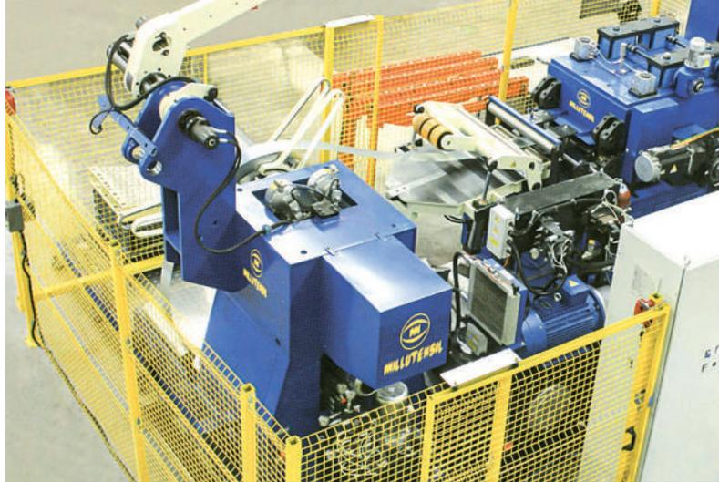
unique in that the automatic production line requires only two people to run. The high productivity is ensured by this rolling-feeder. Moreover, the metal thickness may be anywhere between 0.5 mm to 10 mm.
